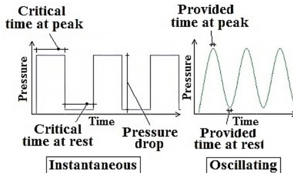
Fig. 27 Critical and provided times at peak and rest during the oscillating and instantaneous variable pressures
