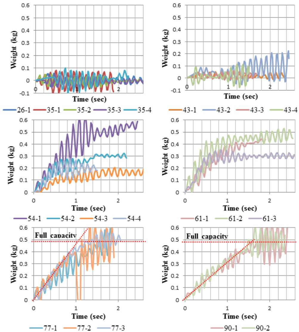
Fig. 18 Penetrability evaluated using OFP with 26-90  $\mu\text{m}$  filters using the weight-time measurement
