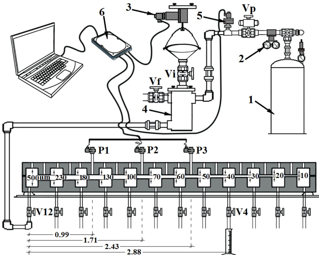
Fig. 43 Schematic view the test set-up: 1) gas tank, 2) pressure regulator, 3) load cell, 4) grout tank, 5) pressure sensor, 6) DAQ – data acquisition system
