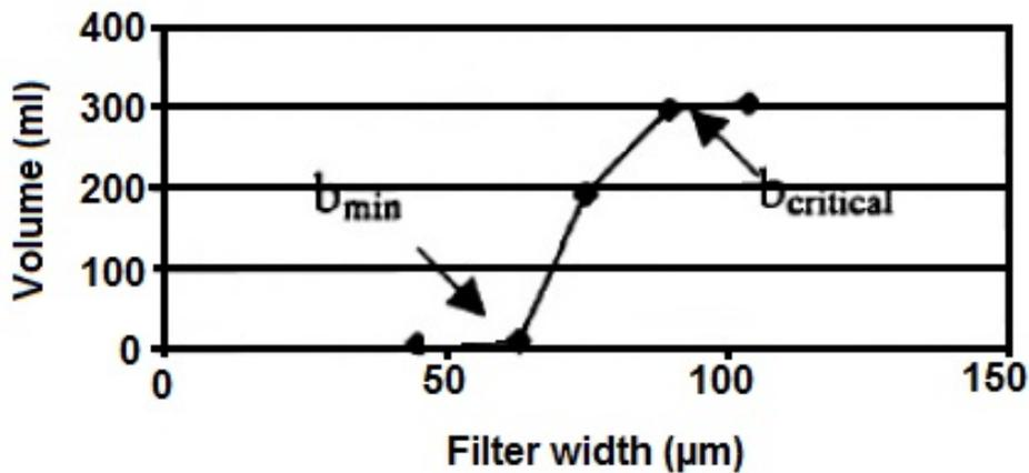
Fig. 5 Evaluation of  $b_{min}$  and  $b_{crit}$  according to Eriksson et al. (2000)
