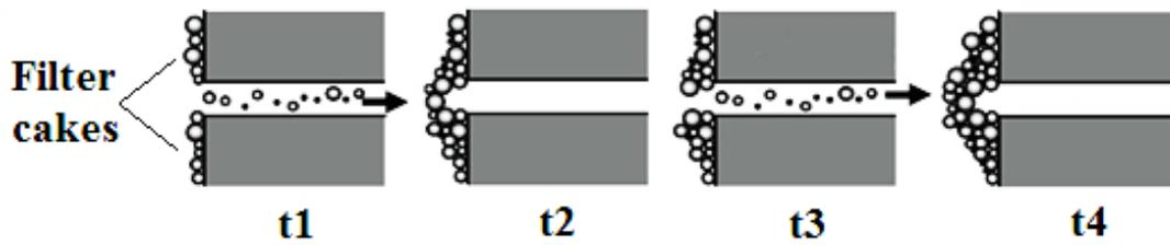
Fig. 9 Filtration process suggested by Nobuto et al. (2008)
