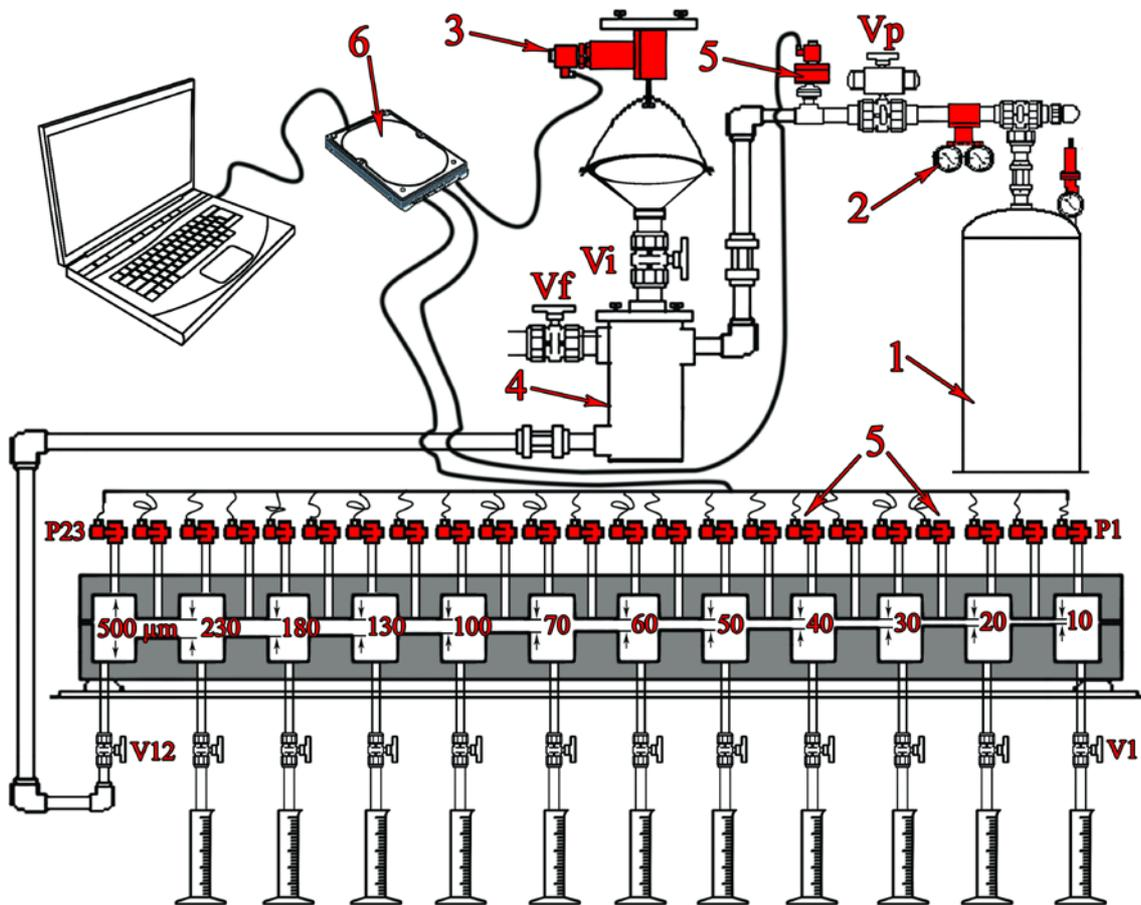
Fig. 22 Schematic view of VALS: 1) gas container, 2) pressure regulator, 3) load cell, 4) grout tank, 5) pressure transducers, 6) DAQ
