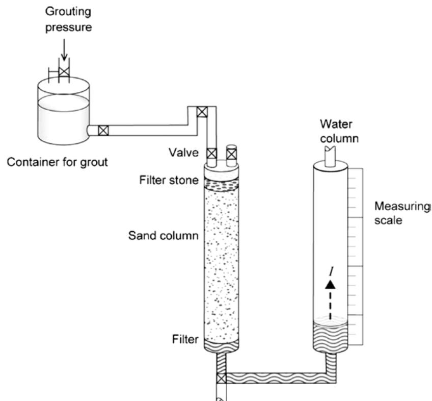
Fig. 1 Schematic view of Sand column according to Axelsson et al. (2009)
