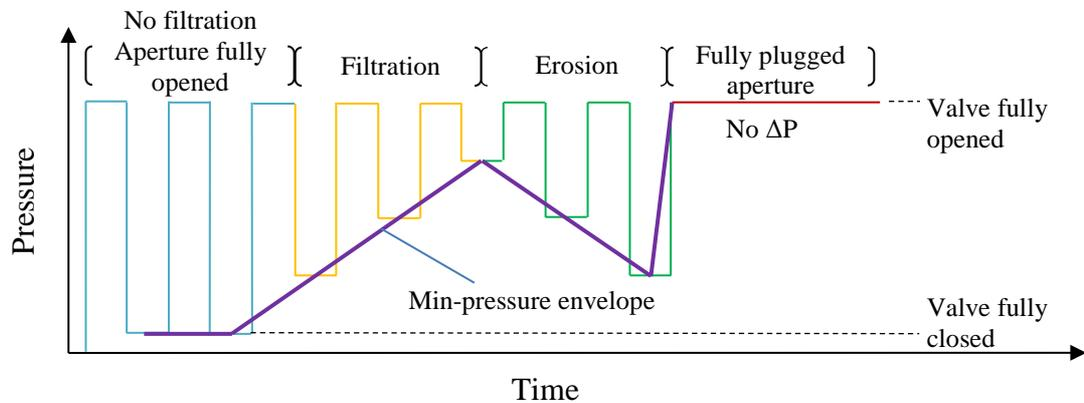
Fig. 30 Use of min-pressure envelope to visualize the filtration and erosion processes
