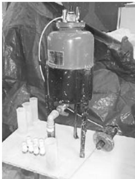
Fig. 6 Penetrability meter developed by Eriksson and Stille (2003)
