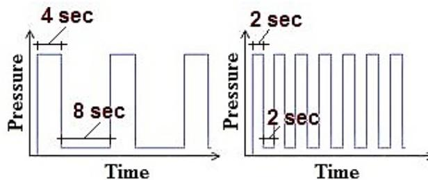
Fig. 28 Instantaneous variable pressure with peak/rest periods of 4 s/8 s and 2 s/2 s
