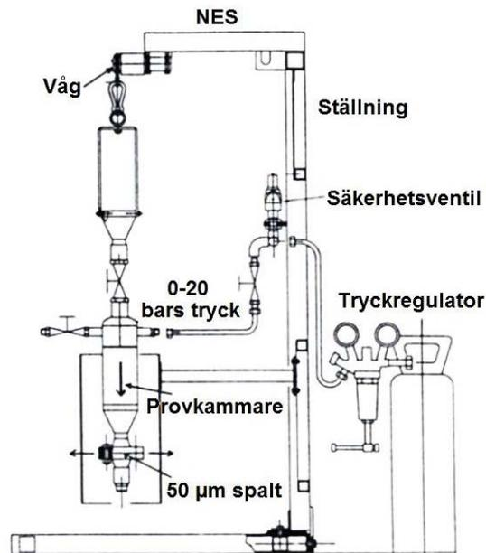
Fig. 8 Schematic view of NES method (Sandberg, 1997)
