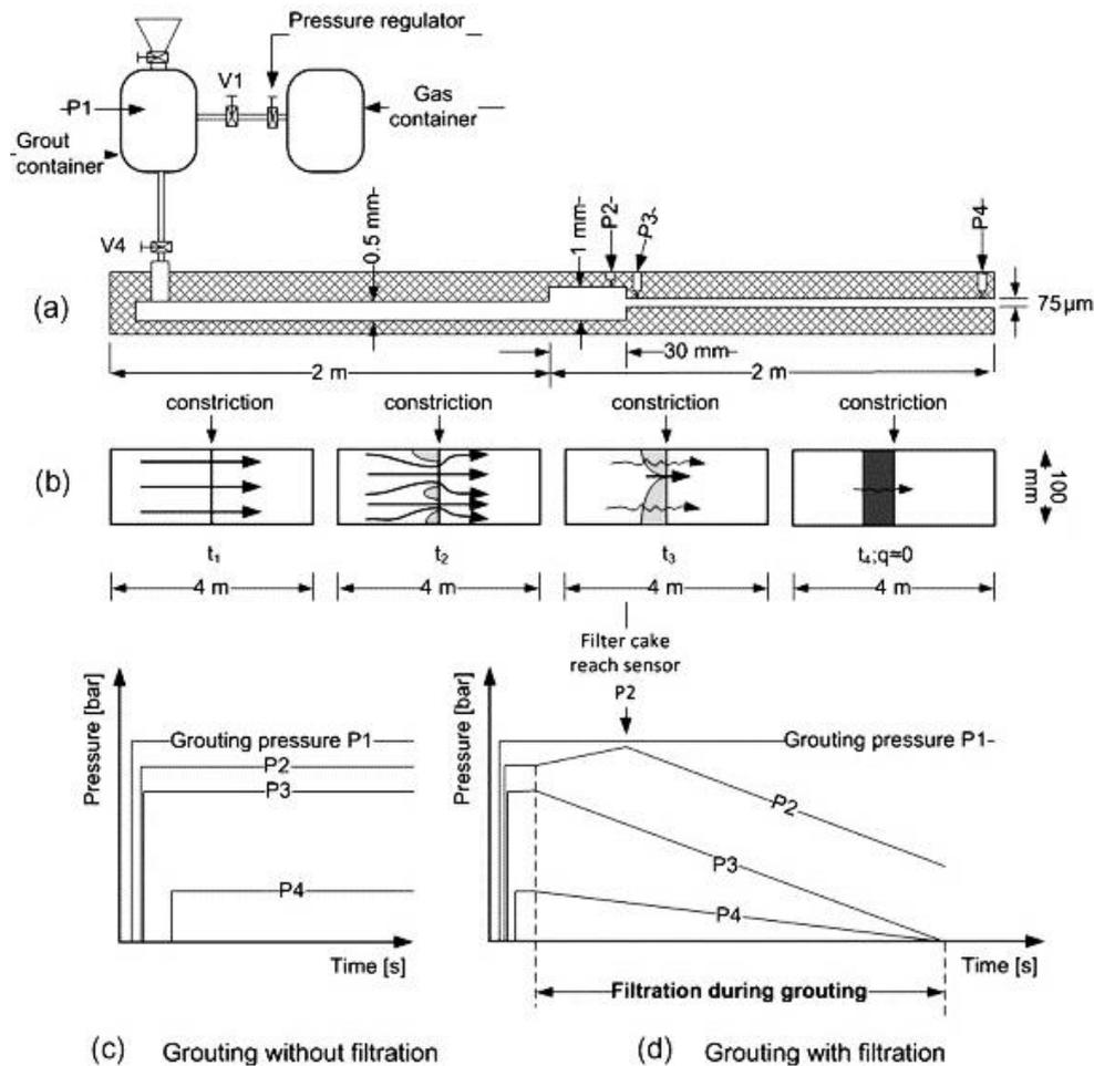
Fig. 12 Cross-section of Long slot (a), process of plug formation at the constriction (b) and pressure variation along the slot with and without filtration (c) and (d), respectively (Draganovic and Stille 2014)
