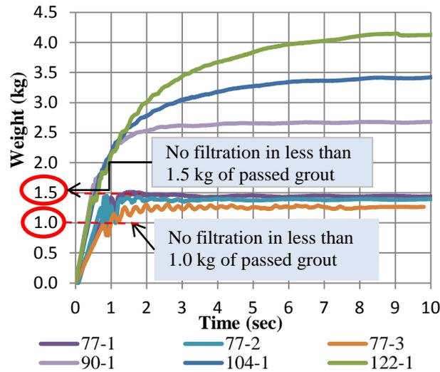
Fig. 20 Penetrability evaluated using MPM with 77-122  $\mu\text{m}$  filters using the weight-time measurement
