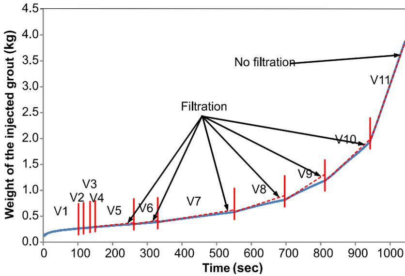
Fig. 24 Monitoring the filtration process in test G1-T1
