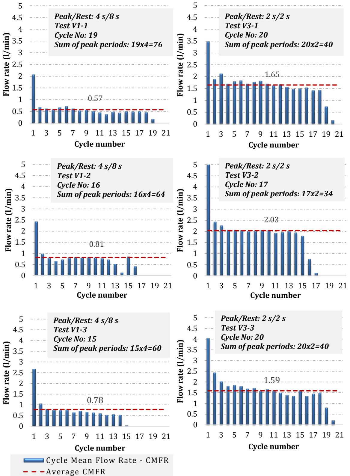
Fig. 32 Cycle mean flow rates (CMFRs) and average CMFRs for the experiments using 43- $\mu$ m slot with 4 s/8 s and 2 s/2 s peak/rest periods
