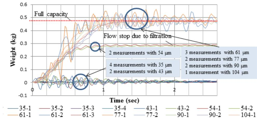
Fig. 19 Penetrability evaluated using MFP with 35-104  $\mu\text{m}$  filters using the weight-time measurement
