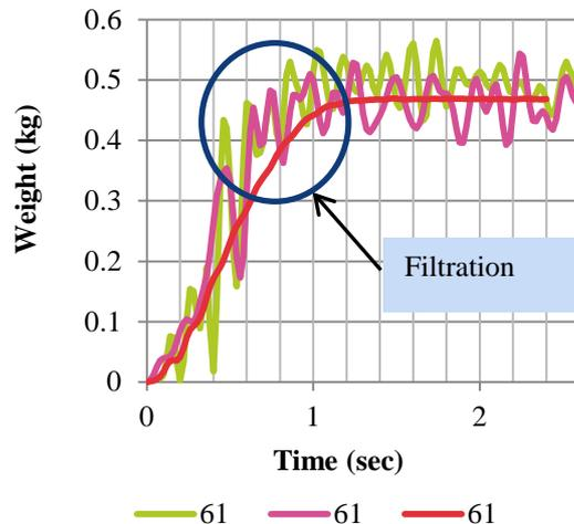
Fig. 21 Penetrability evaluated using MFP with  $61\text{-}\mu\text{m}$  filter using the weight-time measurement
