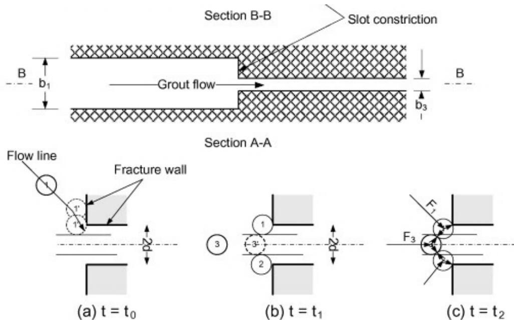
Fig. 11 Cross-section of Short slot (upper) and arching of the cement particles over time (lower) (Draganovic and Stille 2011)
