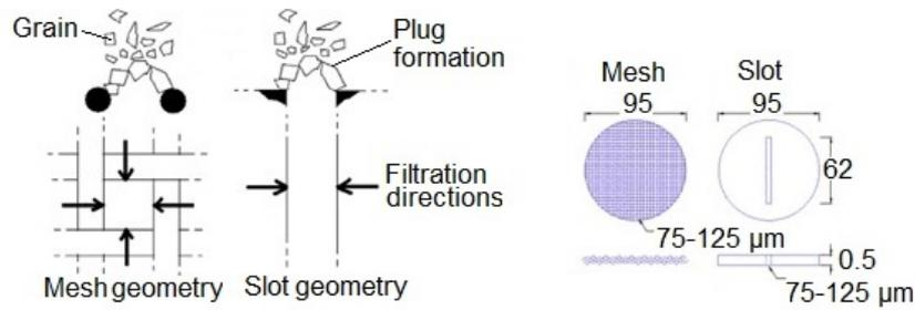
Fig. 7 Mesh and slot geometries in penetrability meter (Eklund and Stille, 2008)
