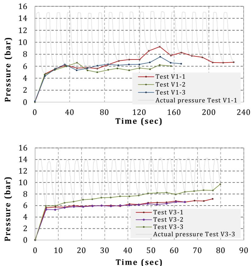
Fig. 31 Min-pressure envelopes obtained using 43- $\mu\text{m}$  slot with 4 s/8 s (top) and 2 s/2 s (bottom) peak/rest periods
