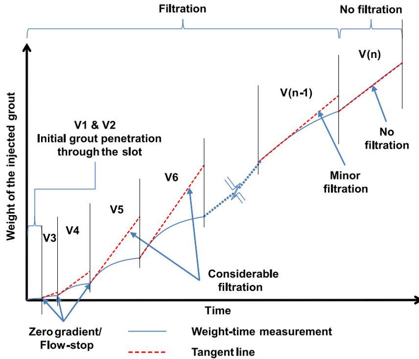
Fig. 23 Monitoring the filtration using the weight-time measurement
